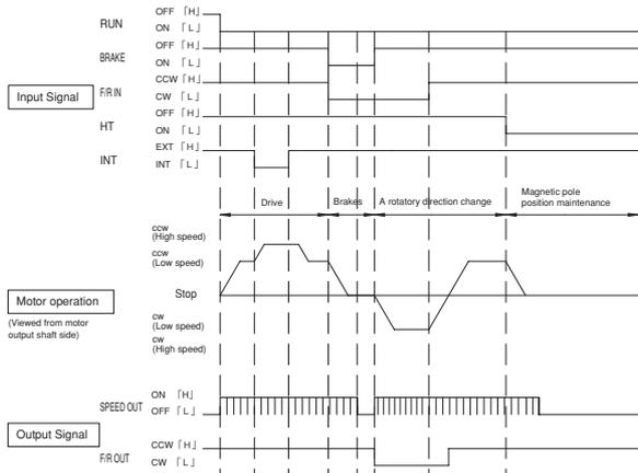
The INT signal is the signal that switches internal speed specified voltage and external speed specified voltage. In this control sequence, the voltages are set up as internal speed voltage for low speed and external speed voltage for high speed operation.
