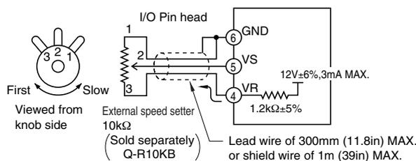
Fig.2 Speed setting by external voltage supply
