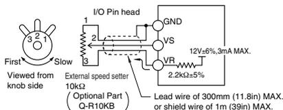
Fig.2 Speed setting by external voltage supply
