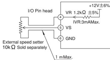
Fig.2 Speed setting by external voltage supply
