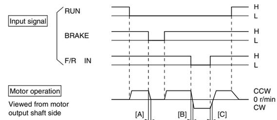
[Notes for "BRAKE" operation and during the rotation direction changing] "BRAKE" (Above [A] period) should be operated, within the "SPEED CONTROL RANGE".
