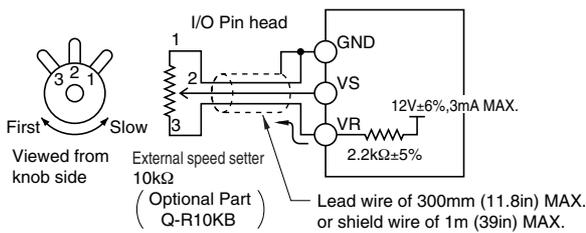
Fig.2 Speed setting by external voltage supply
