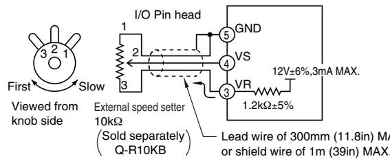
Fig.2 Speed setting by external voltage supply
